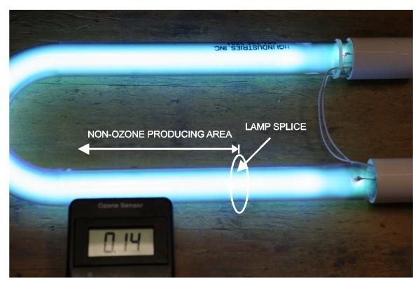
This is a spliced UV lamp where a certain percentage of the lamp is ozone producing and the balance of the lamp is not.
